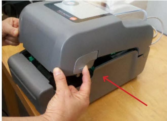
1. Hold down both buttons on either side of the printer then lift the top off.
